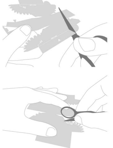
Hint: Sharp folding edges best are obtained when, before folding, you slightly carve the lines either with a knife (just dent, don't cut) or with the point of your scissors. Careful. Just dent enough so the paper 'knows' where it needs to bend.
